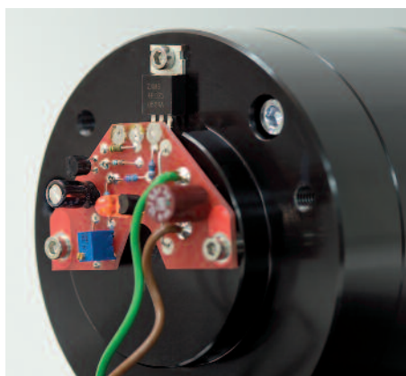
The “Balance” MOS-FET bearing heater assembly
